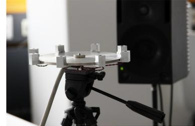
Figure 2: Microphone array used for measuring RIRs.
